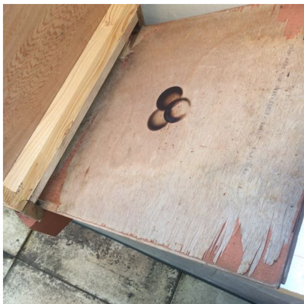
Heat shield (showing burn marks from previous use).
