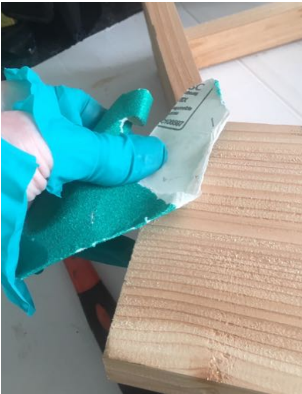
Sanding the corners so the panel slots in.
