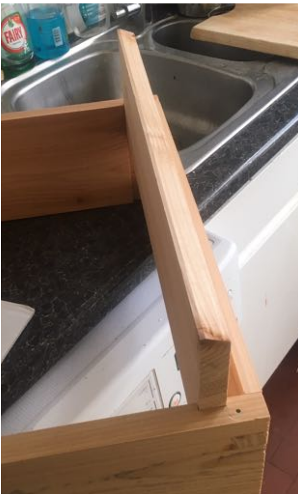
Slotting in the side panels
