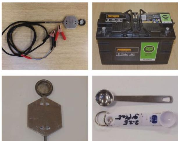
(Top left) VarroX® sublimator, 12v and 150 W. (Lower left) Close-up of the heated cup at the end of the sublimator into which the oxalic acid crystals are placed. (Top right) Lead-acid battery, 115 Ah, capable of powering the sublimator for approximately seven hours. (Lower right) Half-teaspoon measures are cheap to buy and are a convenient way of dispensing oxalic acid crystals for sublimation as half a teaspoon, 2.5ml, of oxalic acid crystals is almost exactly 2.25g.
