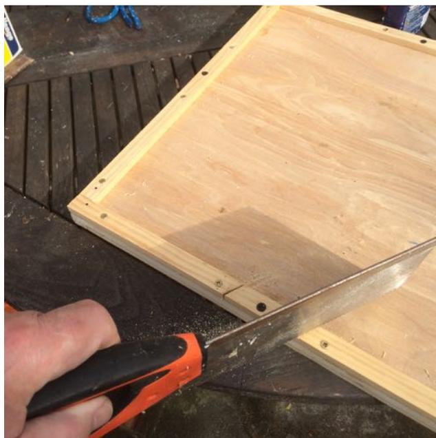
short off-cut of the strip wood and I temporarily nail it to one edge in the corner. Then pin and glue the next strip of wood to one edge at right angles to the temporary. I tend to use 18mm frame pins with Evostick outdoor PVA wood glue, but gorilla glue is better. I then use a handsaw to trim the strip level to the side of board. I then repeat for side two and side three. Once three sides are made, I remove the temporary off-cut and complete side four.
