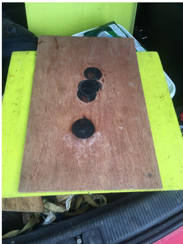
*A plywood board is used to stop the plastic correx inspection board from melting.*
